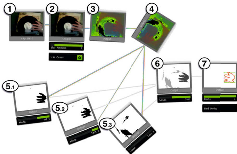
Fig. 6. A Raydiance implementation of an algorithm for hand localization
